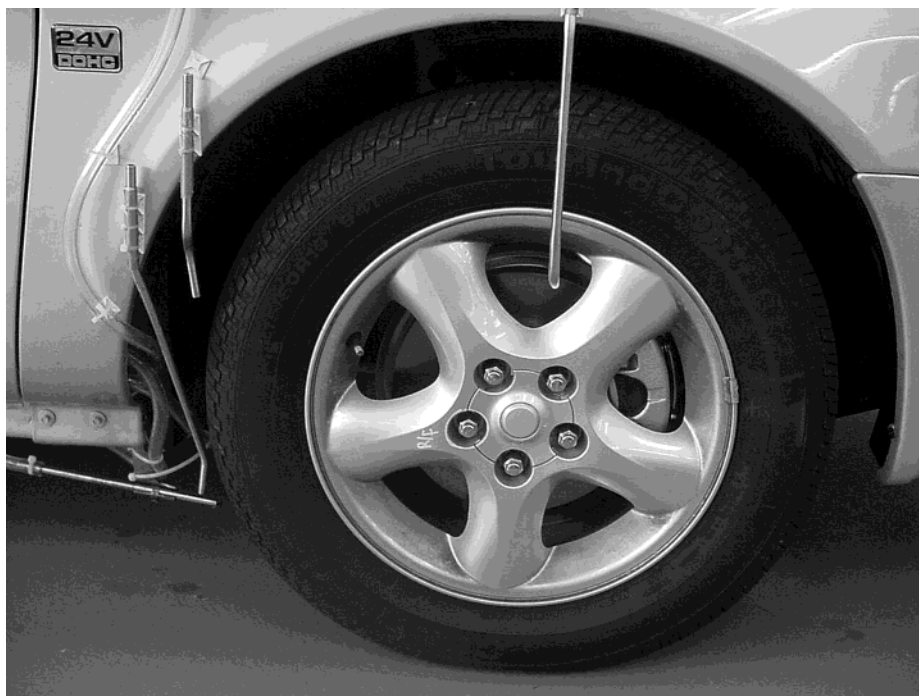
FIGURE 1. Image of test vehicle showing location of sampling tubes. All positions shown, including a longer vertical tube reaching to the center of the wheel, were tested. The three positions were (i) along the wheel centerline extending to the cut-outs in the wheel covers (shown), (ii) at the axle (not shown), and (iii) in the wheel well behind the tire.
