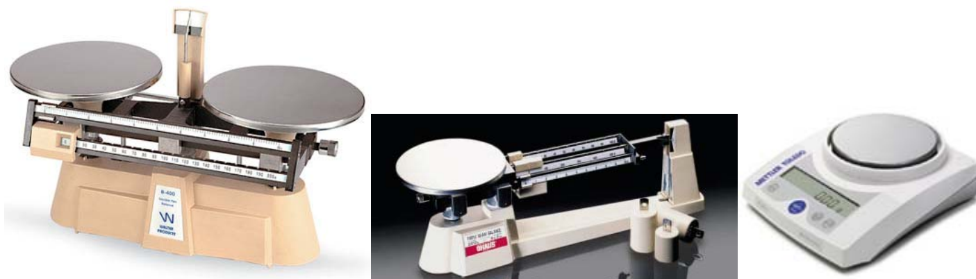
Figure 1.2 Laboratory balances. (a) A double-beam, double platform (pan) Harvard trip balance, which is also called an equal-arm balance . (b) A single platform, triple-beam balance. (c) A digital electronic balance.
